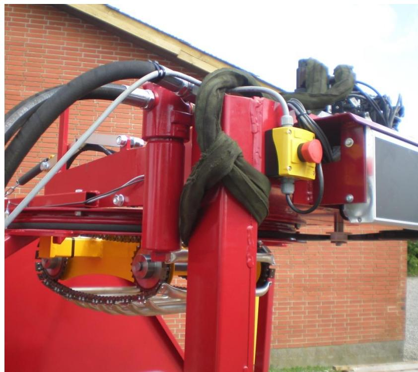
If you need to lift the wrapper using a crane, mount the straps as shown in the illustrations. In this position the machine is in a reasonable state of equilibrium.
